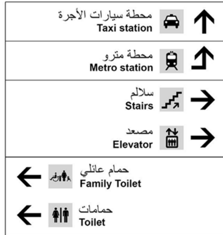
Figure B.104 Examples of directional signs with the correct alignment and hierarchy of arrows
