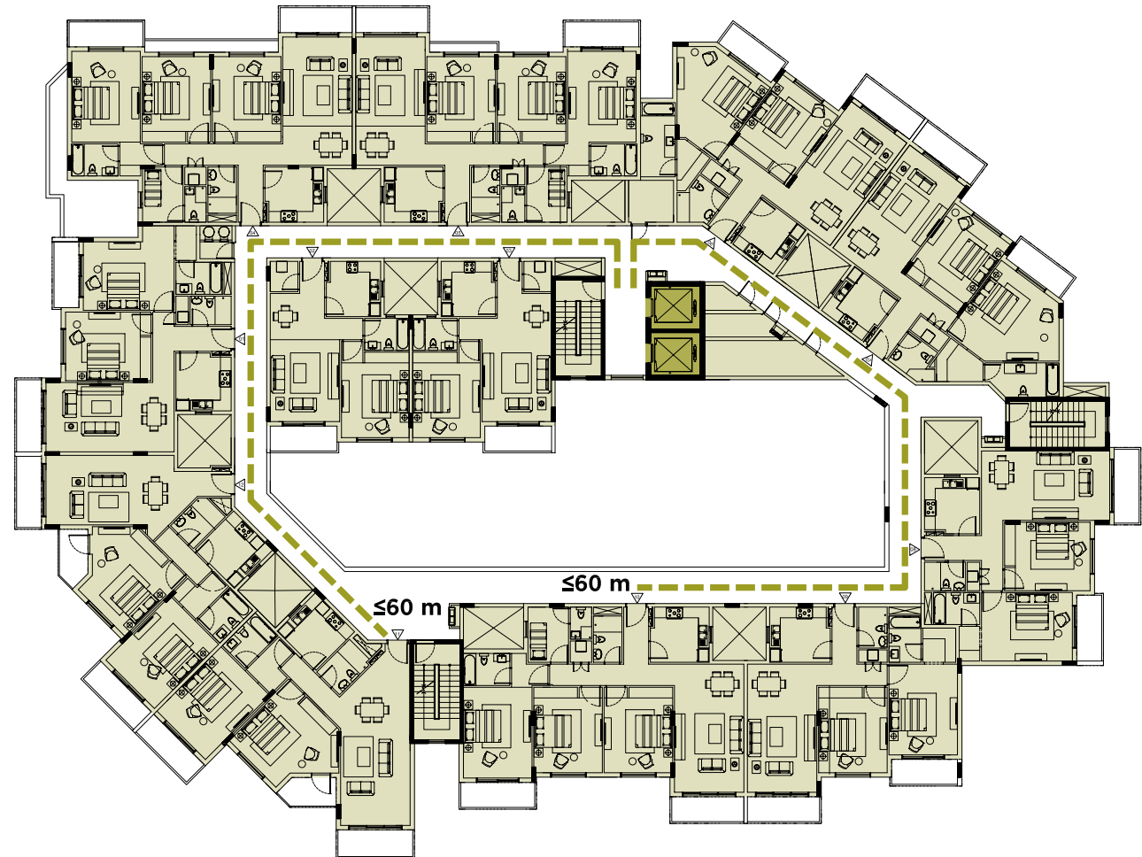
Figure D.3 Floor plan with elevator lobby showing maximum travel distance to an elevator
