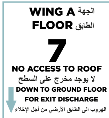
Figure B.36 Example stair signage
